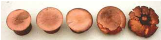
Figure 1. Deformation of copper cylinders exposed to different intensities of shock wave effects (the boundary deformation is marked)
