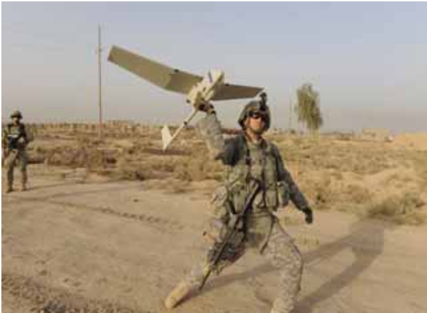
Figure 5. A soldier is launching the most numerous UAV in the US Army - AeroVironment RQ-11B Raven, intended for observing and reconnaissance [28]
