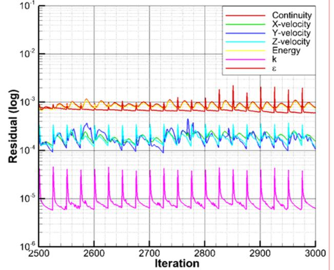
Figure 10. Residual versus iteration for the unsteady solution
