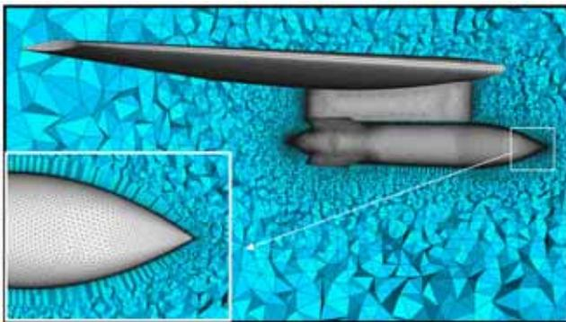
**Figure 6.** Computational grid for the CFD analysis using the NS equation (t=0sec)
