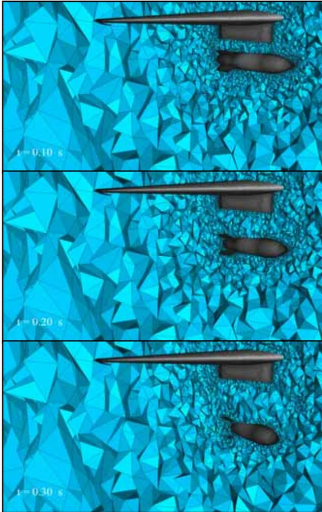
**Figure 5.** Computational grids for the CFD analysis using Euler equations at different time steps
