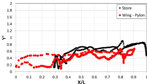
Figure 9.  $y^+$  on the wing-pylon and the store
