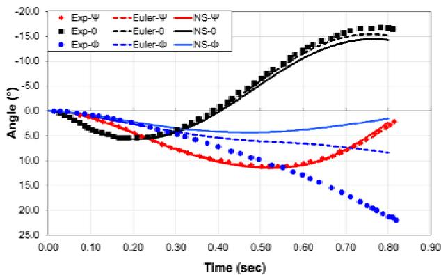
Figure 18. Trajectory of the angular orientation
