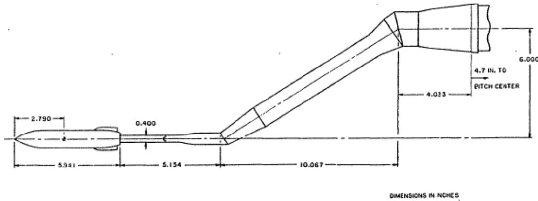
Figure 1. Sketch of the EGLIN test case
