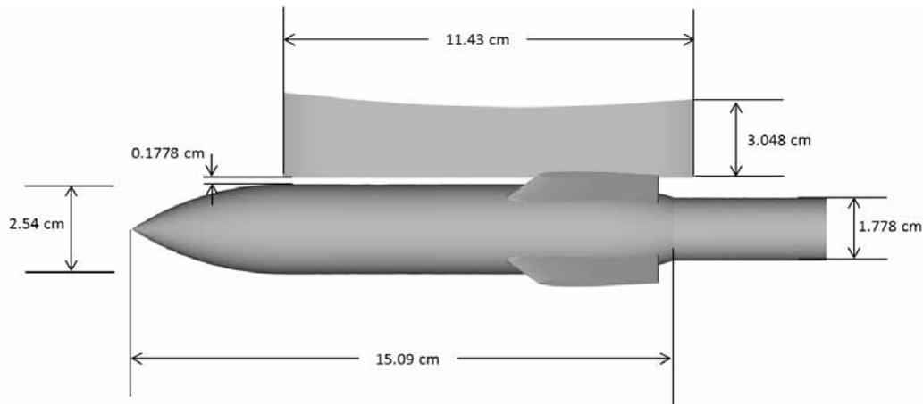
Figure 2. Geometric specifications of the EGLIN test case
