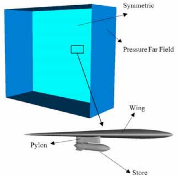
**Figure 8.** Solution domain and a part of the EGLIN test model
