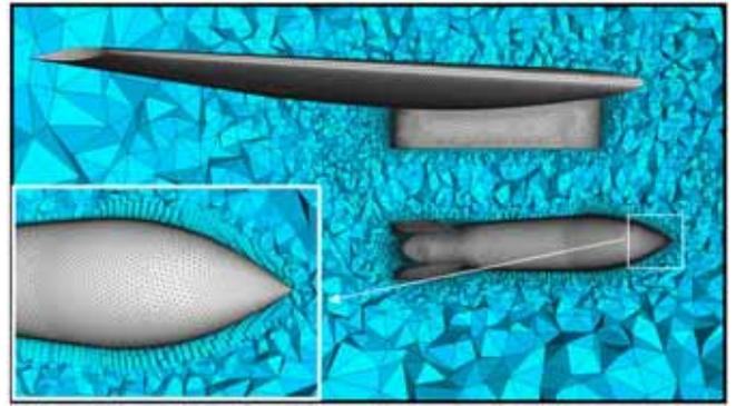
**Figure 7.** Computational grid for the CFD analysis using the NS equation (t=0.2sec)
