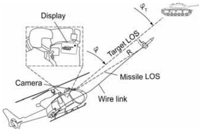
Figure 1. Camera supported manual CLOS guidance
