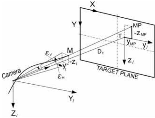
Figure 5. Missile position relative to the LOS.
