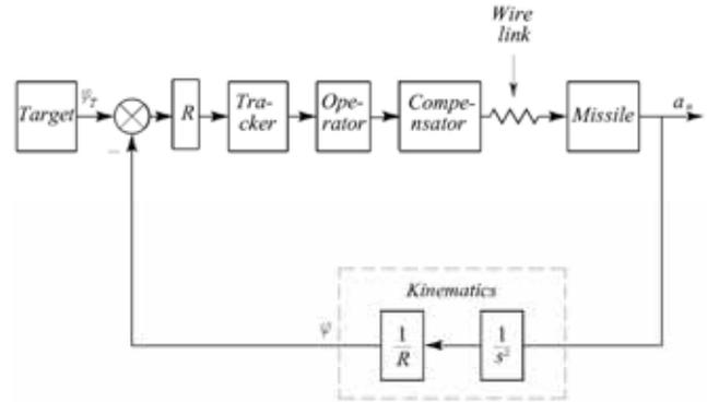
Figure 2. Block diagram of a manual CLOS guidance closed loop.
