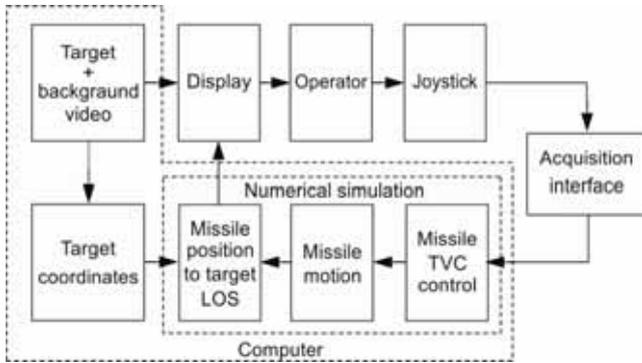
Figure 4. Training simulator block diagram.
