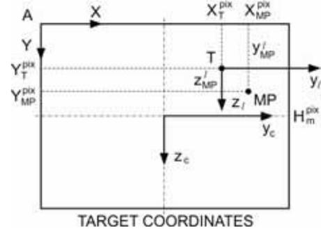
Figure 7. Target and missile silhouette in the video-frame axis system.
