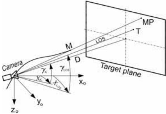
Figure 3. Image formation on the target plane.
