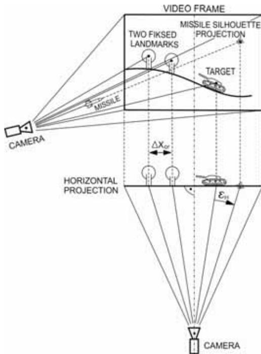
Figure 6. Landmarks and target position in the video frame.
