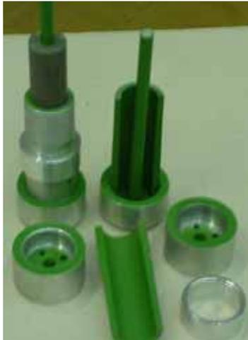
**Figure 5.** Casting tools for ballistic determination
