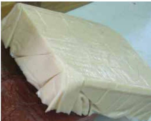
**Figure 6.** Propellant after a curing period
