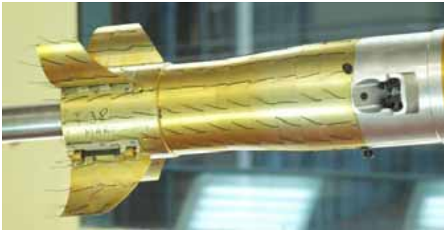
Figure 18. Flow visualization around the ATM model rear section at M = 0.2 , \alpha = 6^\circ and \phi' = 0^\circ , with jets, lower tabs in the jets
