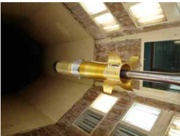
Figure 3. The ATM model on the MSS in the T-35 wind tunnel, \phi = 90^\circ
