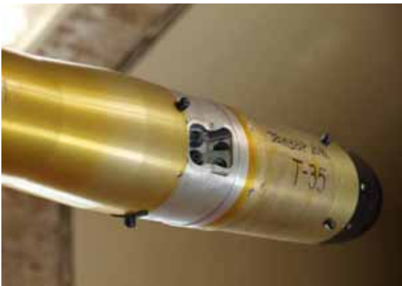
Figure 2. The ATM model on the MSS in the T-35 wind tunnel, \phi = 0^\circ
