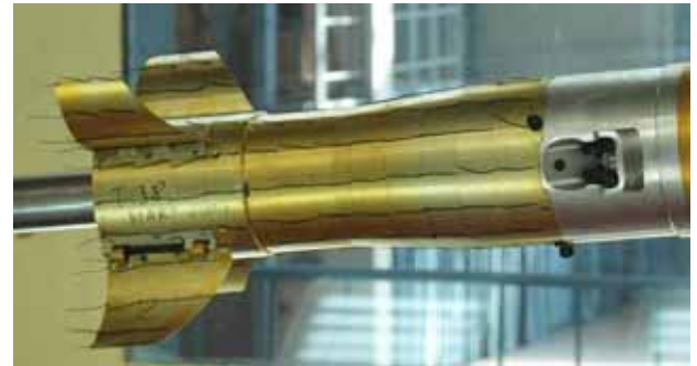
Figure 15. Flow visualization around the ATM model rear section at M = 0.2 , \alpha = 6^\circ and \phi' = 0^\circ , without jets
