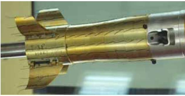
Figure 17. Flow visualization around the ATM model rear section at M = 0.2 , \alpha = 6^\circ and \phi' = 0^\circ , with jets, upper tabs in the jets
