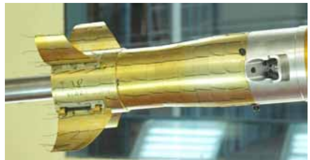
Figure 16. Flow visualization around the ATM model rear section at M = 0.2 , \alpha = 6^\circ and \phi' = 0^\circ , with jets, tabs out of the jets
