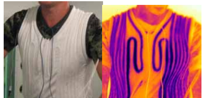
Figure 5. Vest snapshot recorded with a standard (a) and a thermal imaging camera (b), in 30th minute of exercise
