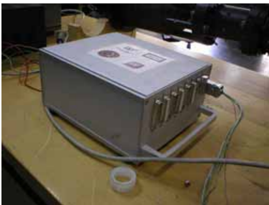
Figure 7. Control box of the flow cell
