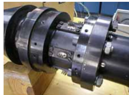
Figure 4. Details of the total pressure rake at the engine face, inside a, b), and details outside c)
