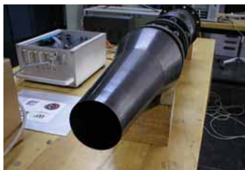
Figure 9. The flow cell with the Pitot air intake in the T-38 wind tunnel test section a) and Pitot air intake b)
