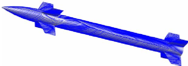
**Figure 14.** Surface Streamline Pattern at  $M=1.75$ ,  $\alpha=24^\circ$
