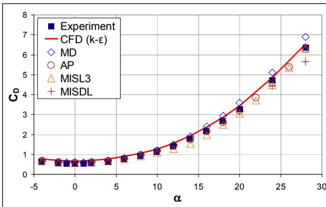
**Figure 19.** Comparison of the experimental drag force coefficient with the CFD and the semi-empirical results at  $M=1.75$
