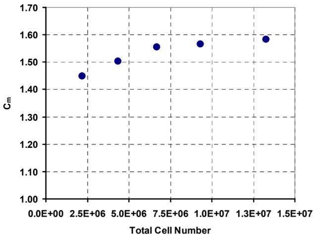
**Figure 5.** The Change of the Pitching Moment Coefficient According to the Total Cell Number
