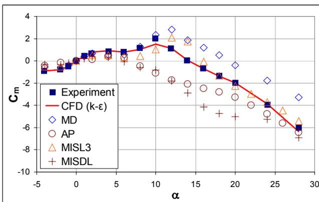
**Figure 20.** Comparison of the experimental pitching moment coefficient with the CFD and the semi-empirical results at  $M=1.75$
