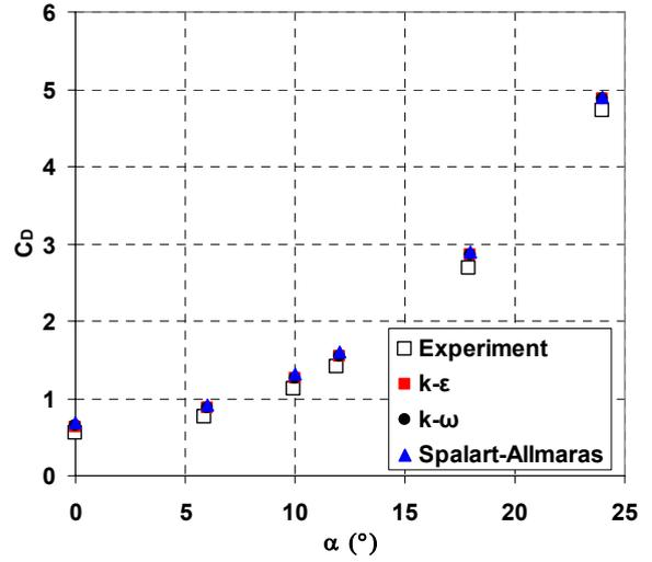
Figure 10. Drag Coefficient Comparison
