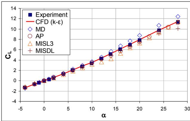
**Figure 18.** Comparison of the experimental lift force coefficient with the CFD and the semi-empirical results at  $M=1.75$
