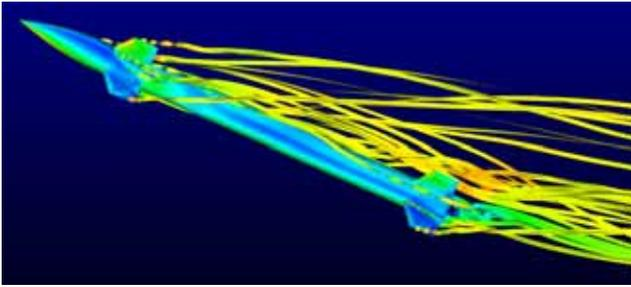
**Figure 13.** Pressure Contours and Streamlines at  $M=1.75$ ,  $\alpha=24^\circ$
