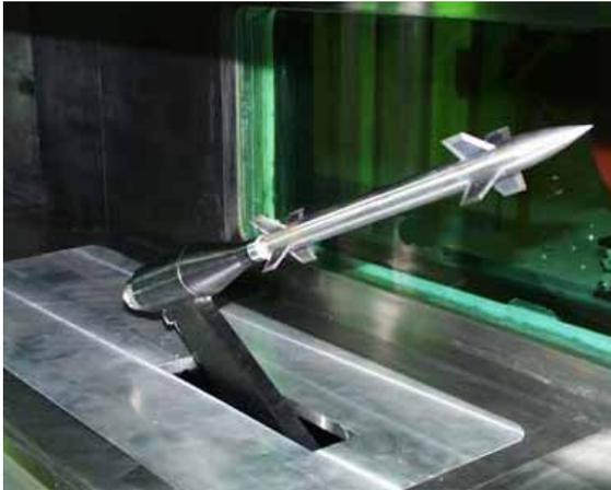
Figure 2. Small-scale NTCM Model [1]
