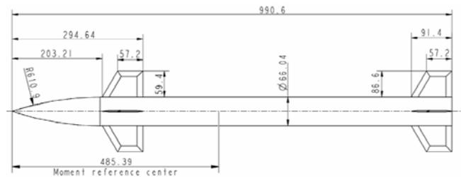
Figure 1. NTCM Configuration (all dimensions are in millimeters)
