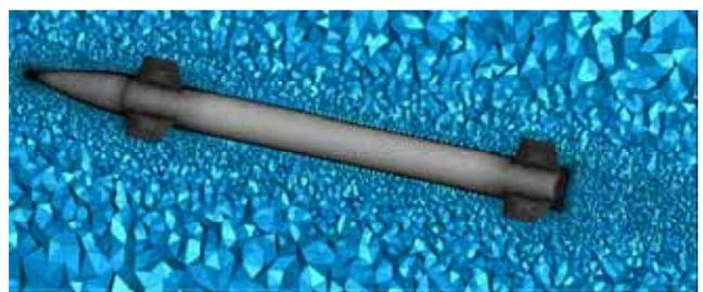
**Figure 8.** Cross Sectional View of the Computational Domain
