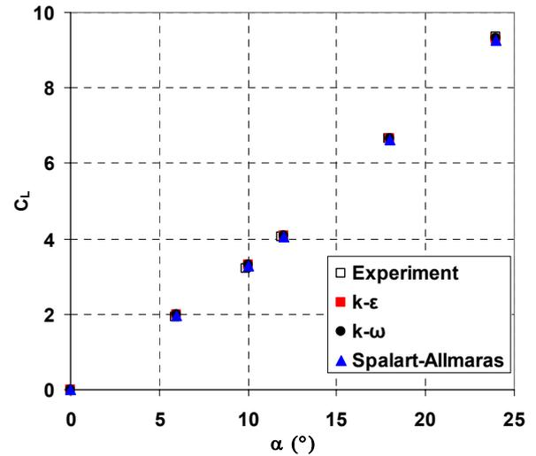
Figure 11: Lift Coefficient Comparison
