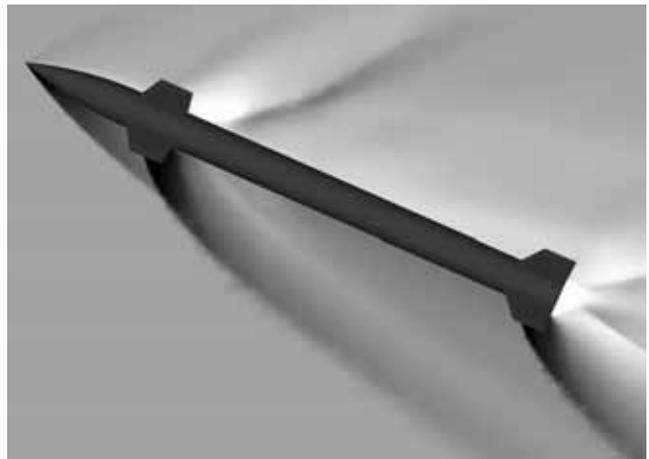
**Figure 17.** Shock Wave Visualization,  $M=2.0$ ,  $\alpha=24^\circ$
