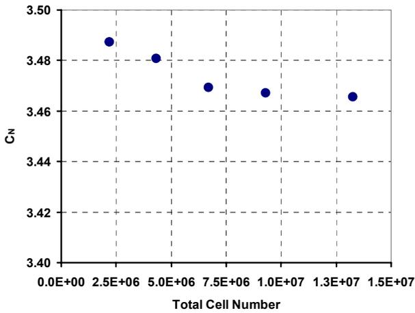
**Figure 4.** The Change of the Normal Force Coefficient According to the Total Cell Number
