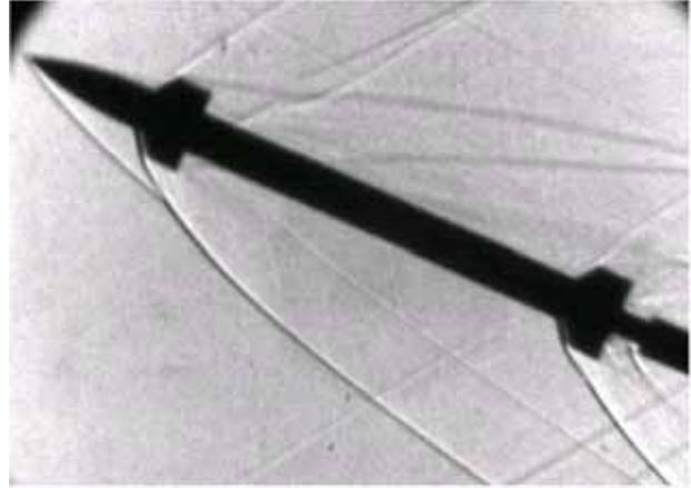
**Figure 16.** Shadowgraph Experiment,  $M=2.0$ ,  $\alpha=24^\circ$  [1]
