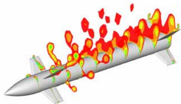
**Figure 15.** Vortices Visualization at  $M=1.75$ ,  $\alpha=24^\circ$
