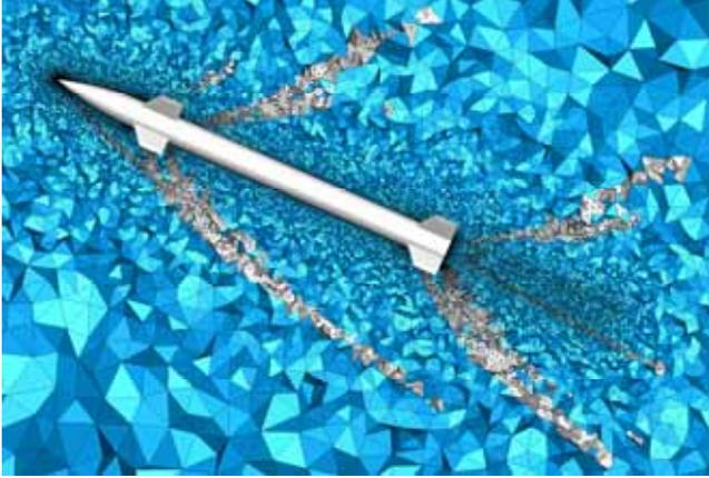
Figure 9. Adapted Grid for the Small-scale NTCM Model (Adapted cells are marked with white)
