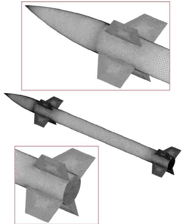
**Figure 7.** Surface Grid for NTCM Models
