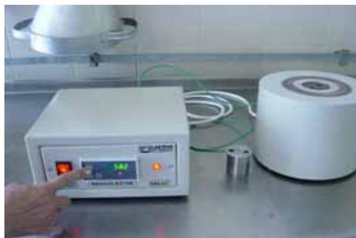
Figure 3. Thermal block with its control unit
