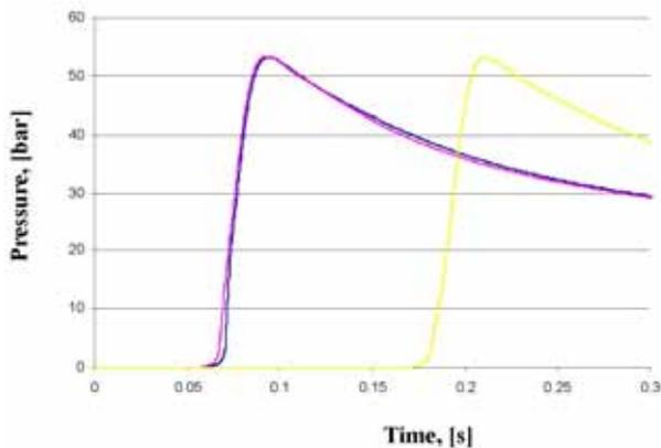
Figure 5. Combustion products pressure vs time diagram – comp 9
