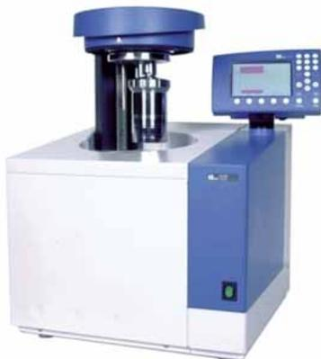
Figure 2. IKA C-2000 Isoperibolic calorimeter
