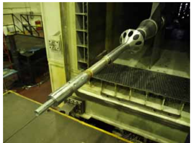
Figure 3. BV40 balance mounted on the sting
