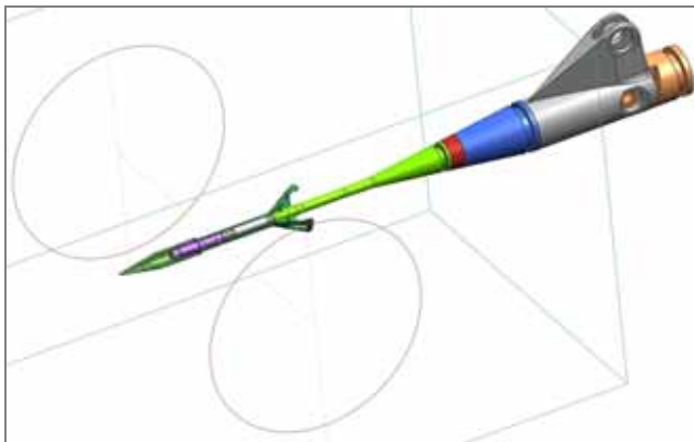
Figure 4. Model position relative to Schlieren windows
