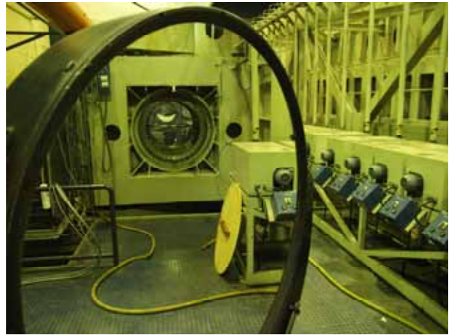
Figure 5. Large diagonal mirror in the T-38 Schlieren system
