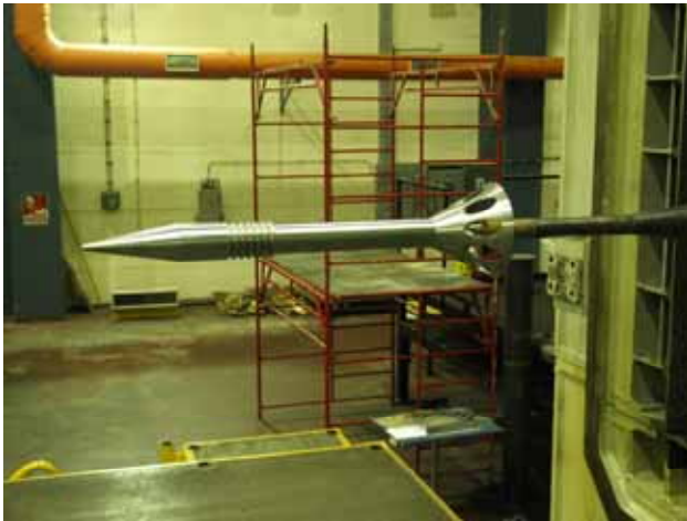
Figure 2. Model of the projectile in the T-38 test section
