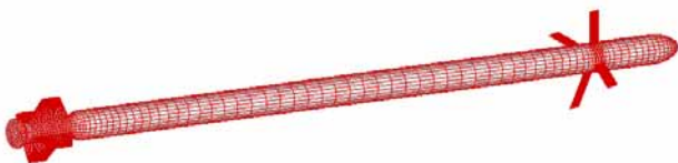
Figure 16. Finite Element Model of the Missile for Structural Analysis
