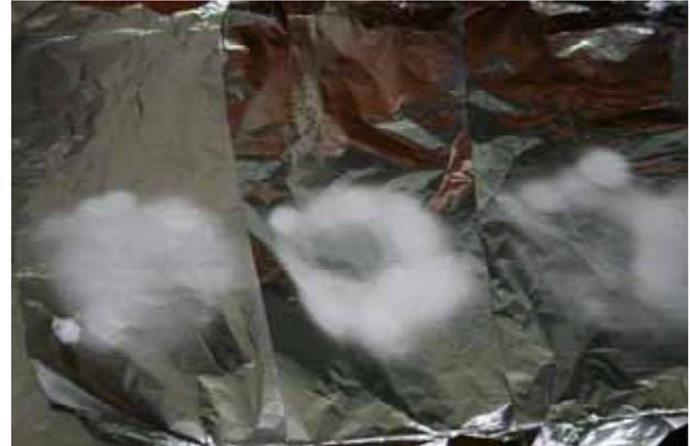
**Figure 4.** The collected nanofibers on the aluminium foils
