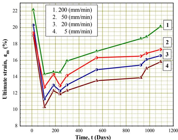
Figure 12. Periodical ultimate-strain results for different crosshead-speeds
