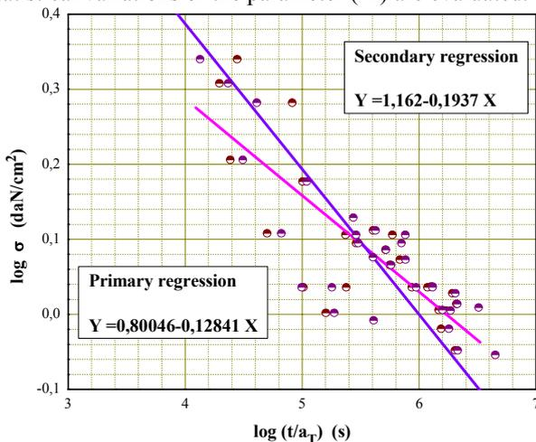
Figure 14. Stress vs Reduced time to failure
