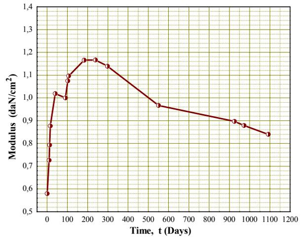
Figure 7. Propellant initial modulus vs time
