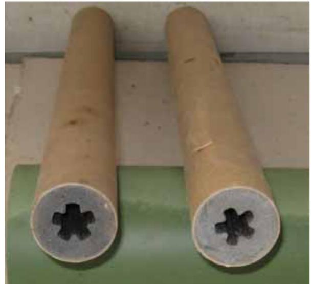
Figure 1. Antihail rocket propellant grain
