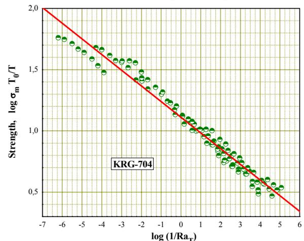
Figure 2. Ultimate stress master curve
