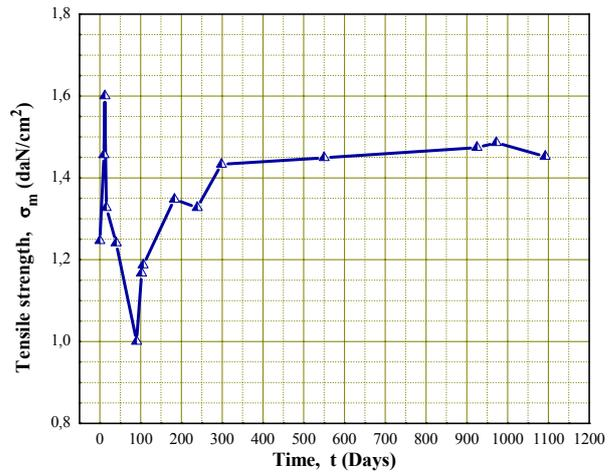
Figure 8. Propellant tensile strength vs time
