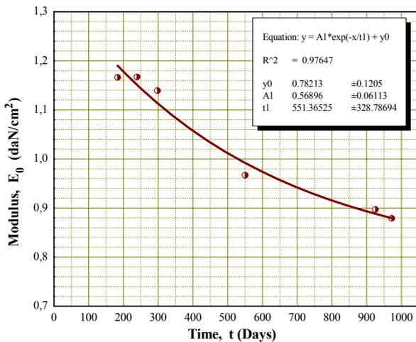
Figure 11. Modulus vs time (2nd phase)
