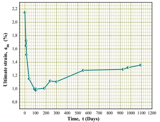
Figure 9. Propellant ultimate strain vs time
