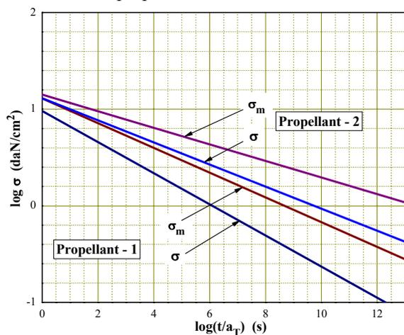
Figure 17. Comparison between ultimate stress ( $\sigma_m$ ) and cumulative damage ( $\sigma$ )
