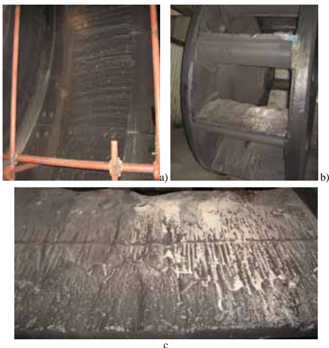
Figure 2. Reconstruction of the ventilation mill:: a-wall plate coating, b-mill wheel and c-impact plate
