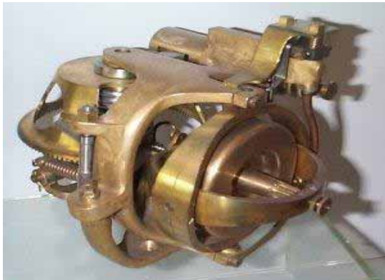
Figure 9. Gyroscope for torpedo stabilization, produced in Germany
