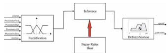
Figure 10. Block scheme of the FIS developed for obstacle avoidance with six input and two output variables
