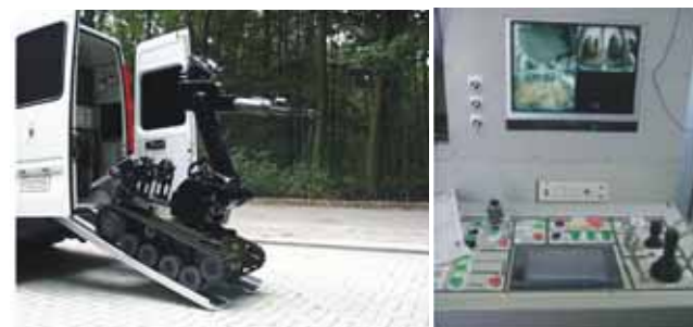
Figure 3. Concept of a remotely supervised mobile robotic system – mobile robot (left) and base-station (right) with a corresponding command and wireless communication interface
