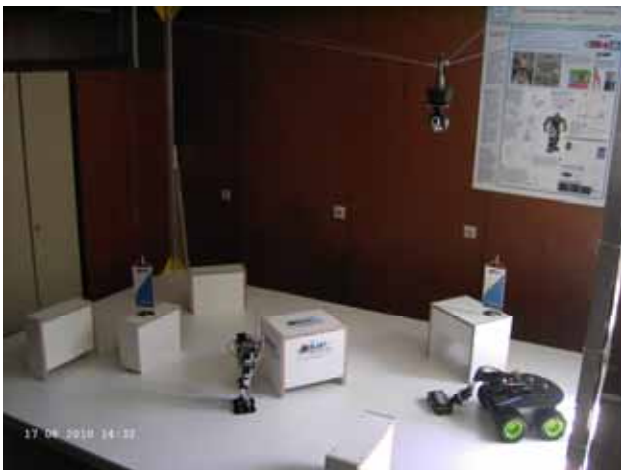
Figure 15. Experimental test-bed station [19] built for research and development of control and navigation of autonomous mobile robotic systems
