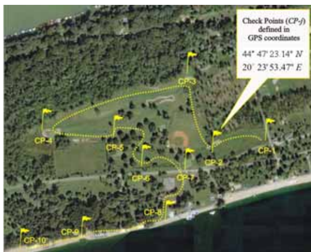
Figure 8. Example of a desired motion of a mobile robot imposed in real outdoor environment by the GPS coordinates of the array of check-points
