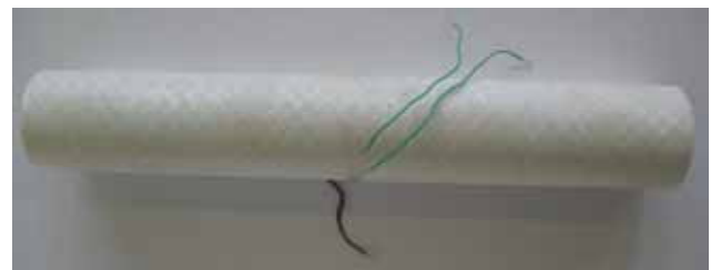
Figure 2. Tube sample with two glued one-axis strain gauges
