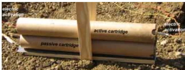
Figure 9. Modified Test 6(a3) applied to the 40 mm L/70 "Bofors" AA gun ammunition with HE-PF projectile
