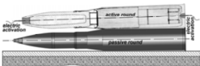
Figure 5. Modified Test 6(a1) applied to the 100 mm T-55 tank gun ammunition with HE projectile
