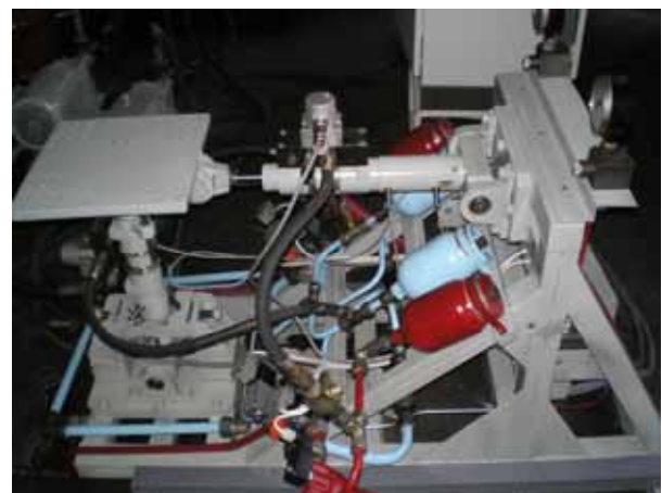
Figure 16. Realized electro-hydraulic vibratory exciter
