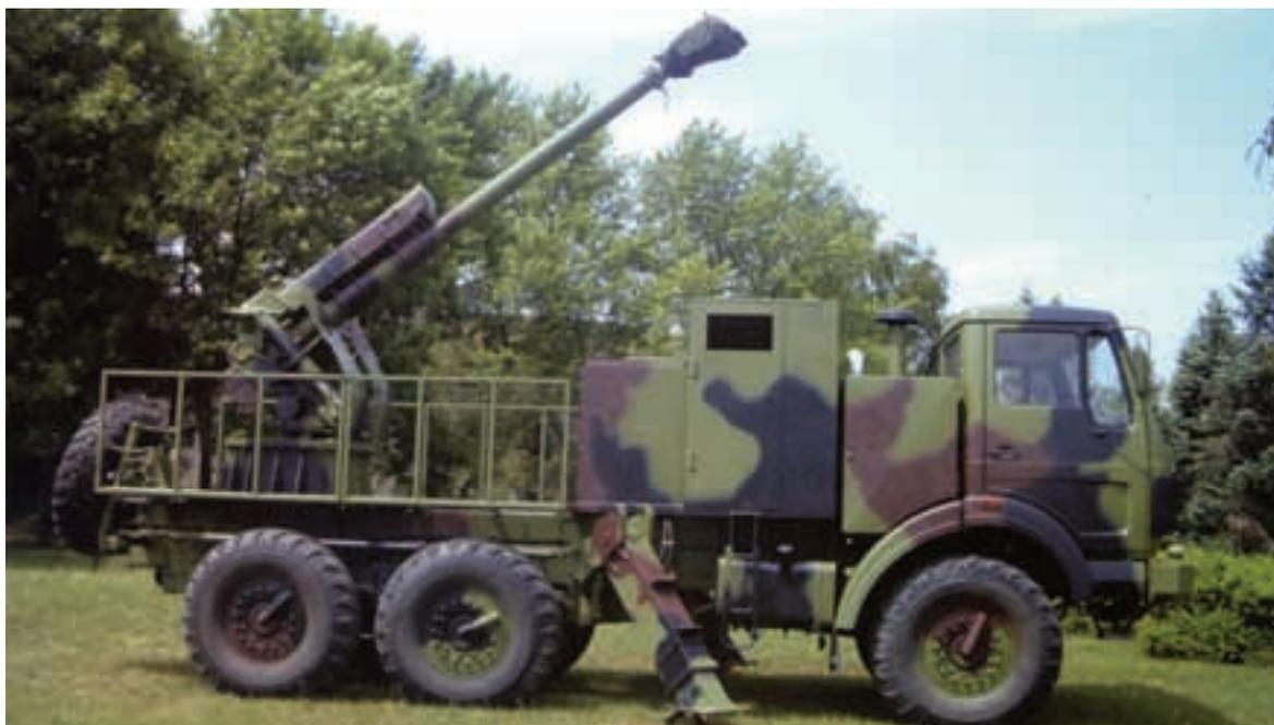
Fig.10. 122 mm self-propelled artillery system SORA
