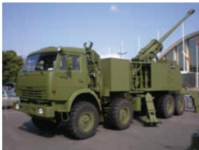
Fig.9. 155 mm self-propelled artillery system NORA-B52
