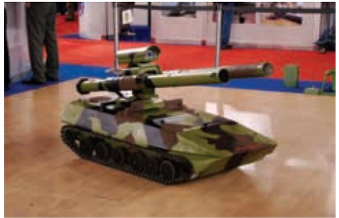
**Fig.16.** MILICA modular robotised anti-armour system
