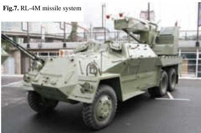
Visitors were also attracted to the modified RL-4M missile system, based on the modification of the R-73 air-to-air IR homing missile and its adaptation to land firing. A booster was fitted in order to compensate for the lacking initial aircraft speed and to achieve a required range. The experts from the VTI and MOMA STANOJLOVIĆ mounted it on the PRAGA vehicle, after removing the turret. This AA technical solution drew the attention of smaller countries in particular due to its affordability.
