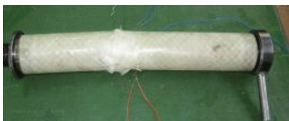
Figure 6. A group A tube after the testing of the internal hydraulic burst pressure
