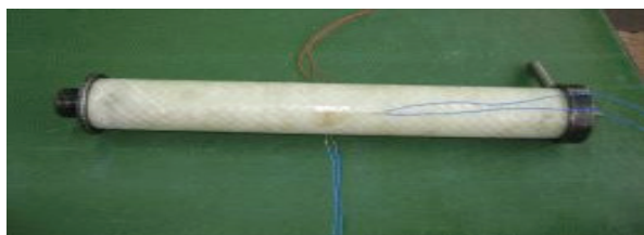
Figure 5. Above mentioned tube sample with glued two-axis strain gauges installed onto the tool for testing the hydraulic burst pressure
