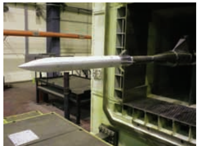
Figure 8. Modified Basic Finner Model in the T-38 test section
