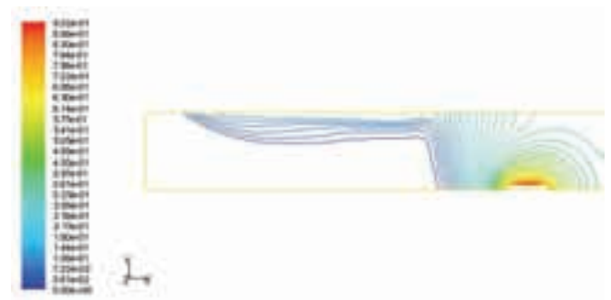
Figure 6. Smoke concentration in the plane of symmetry near the entrance of the tunnel for the adiabatic boundary condition
