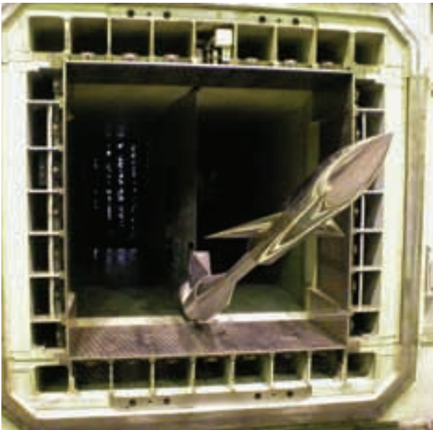
Figure 4. AGARD-B model mounted in the T-38 test section
