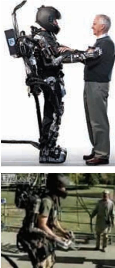
**Figure 1.** Sarcos exoskeleton [5] designed to multiply man power in military tasks
