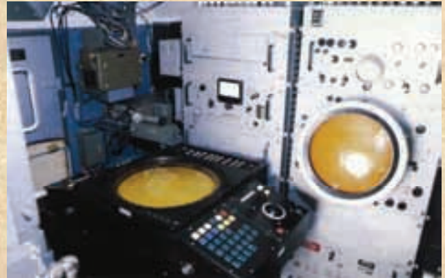
Figure 42. Control board of the surveillance-acquisition radar P-15 in the SONIC system
