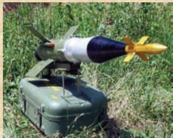
Figure 17. Antitank launching kit MALJUTKA-2T with the tandem warhead
