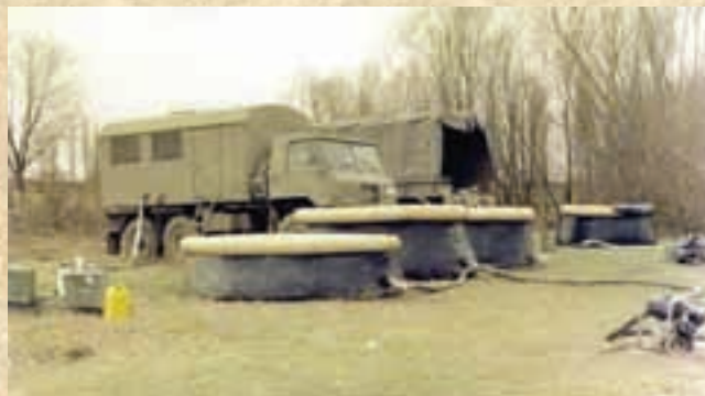
Figure 49. Water station for complex water purification
