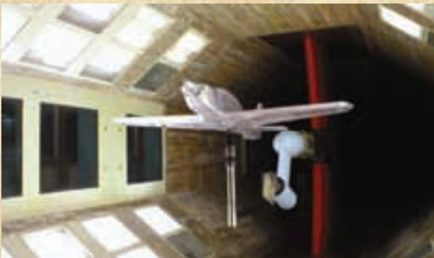
Figure 39. LASTA airplane model in the T-35 wind tunnel
