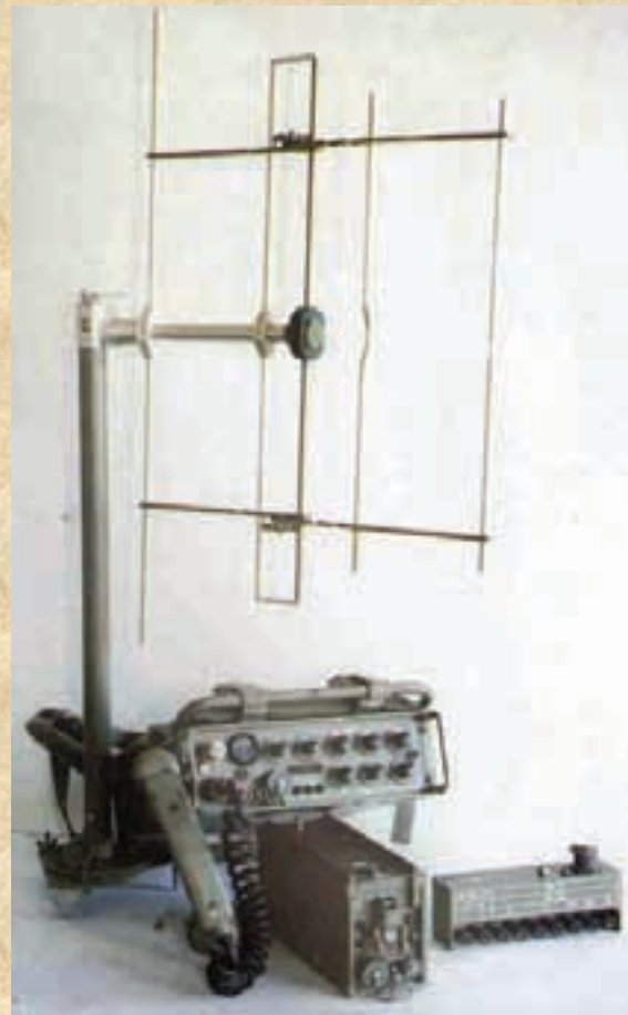
Figure 40. Radio-relay device RRU-1
