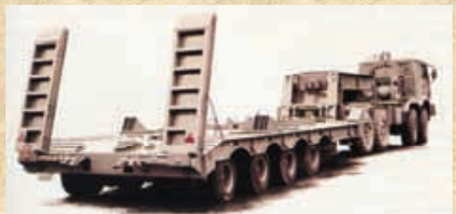
Figure 28. Towed vehicle FAP 3232 with a low-carrying semi-trailer with a capacity of 45 t
