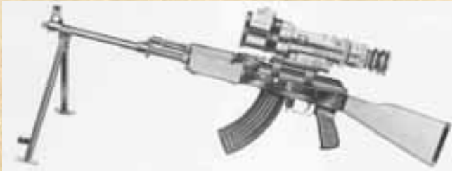
Figure 3. Machinegun M72 with passive night sight
