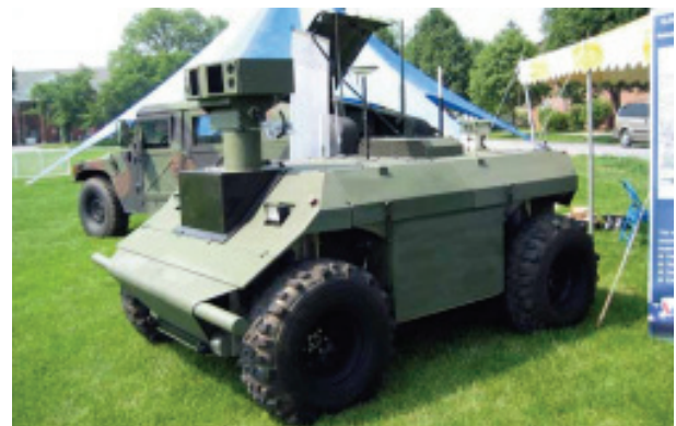
Figure 17. GPS guided, unmanned autonomous, wheel-based, military transport vehicle of the US army
