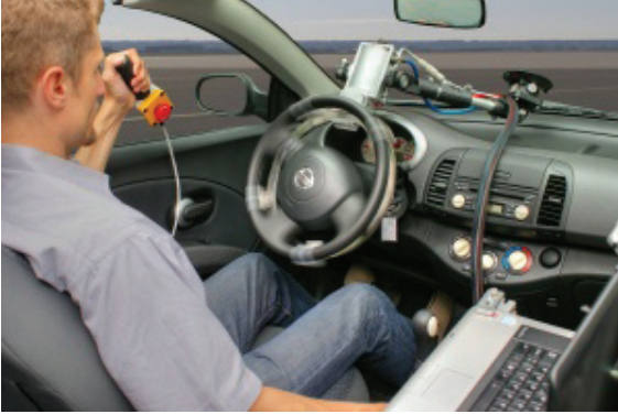
Figure 11. Steering wheel servo actuator [12] assembled to the driver command place
