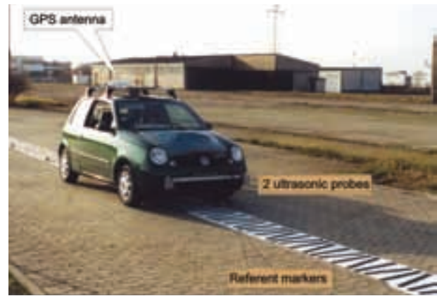
Figure 8. Real-time following path experiments performed by a VW Lupo test-car (TU Braunschweig, IVA, Germany)
