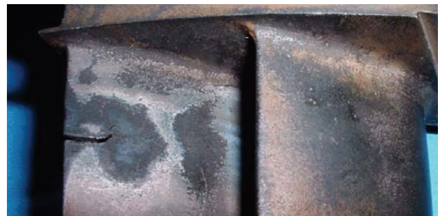
Figure 1. Fracture on the studied blade
