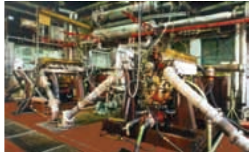
Engine test stands with 1900 kW power rate
