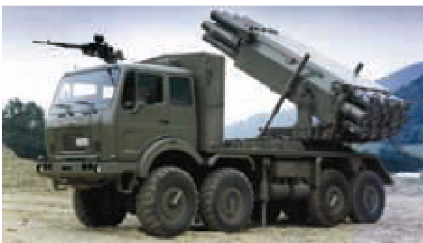
Self-propelled multi-launch rocket system 262 mm M87 "ORKAN"
