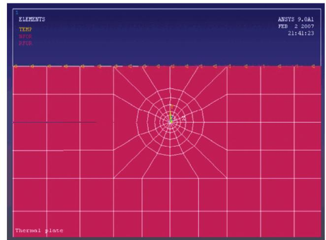
Figure 5. Finite element mesh, close up view around the crack tip
