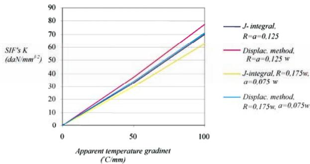
Figure 3. SIFs versus temperature gradients for traction-free boundary conditions
