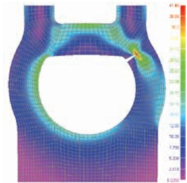
a) crack length of 30 mm
