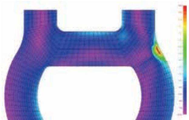
crack length of 60 mm
