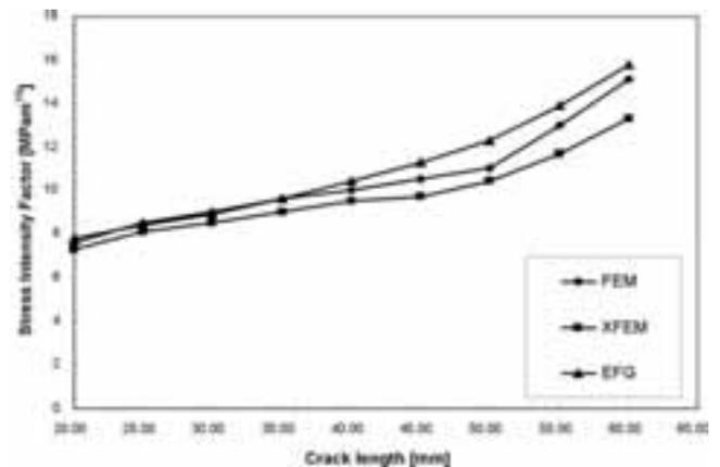
**Figure 5.** Relationship between the stress intensity factor  $K_I$  and the crack length
