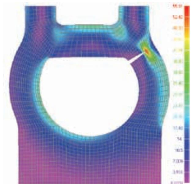
c) crack length of 50 mm
