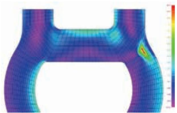
c) crack length of 50 mm
