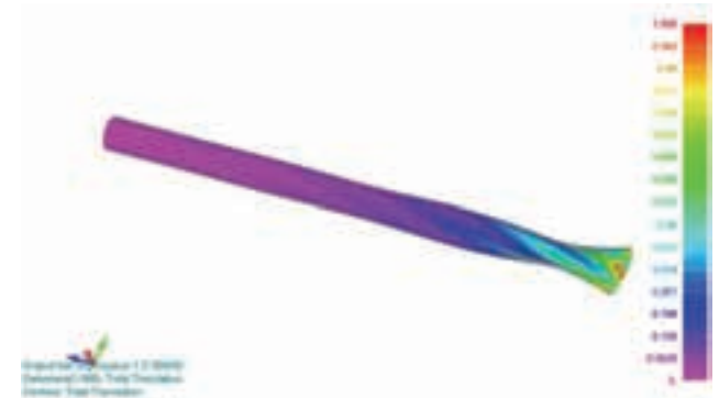
Figure 8. The first mode of torsional buckling of the hybrid aluminum/composite shaft Al/[0 USN,8 ]
