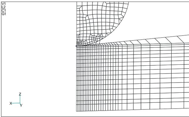
Figure 11. Mesh of finite elements in the contact zone, magnified
