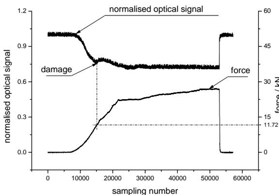
Figure 6. Signal intensity changes during indentation
