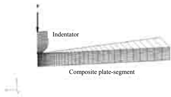
Figure 10. FEM model of the composite segment
