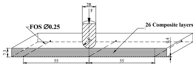
Figure 5. Position of the indenter during testing
