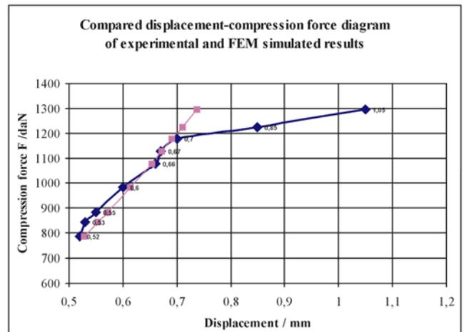
Figure 9. FEM- Experiment displacement vs. compression force results
