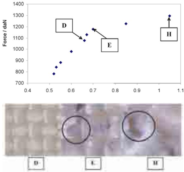
Figure 8. Functional relationships between the indenter displacements and the applied force along with the microscope photos of the characteristic indentation points
