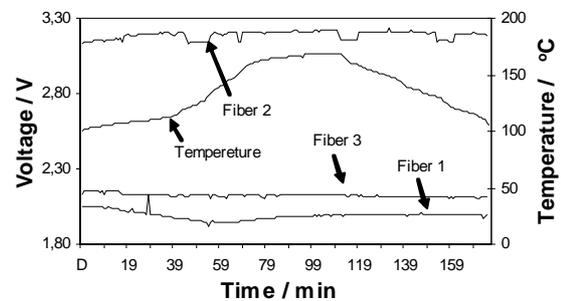
Figure 2. Light signal intensity drop measurement during the optical fibers embedding into the composite material
