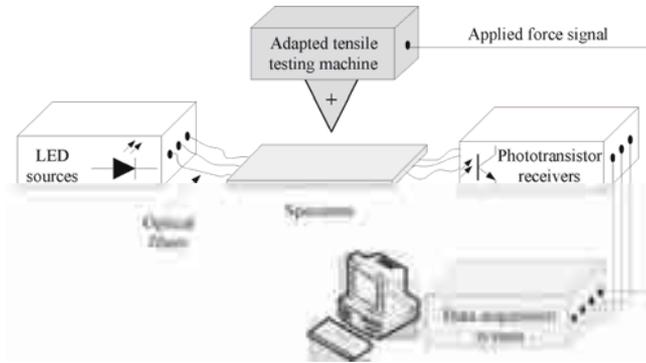
Figure 4. Measuring and acquisition part of the equipment
