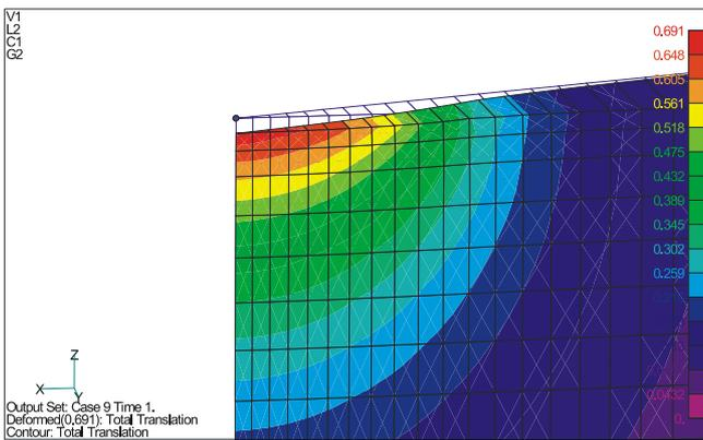
Figure 12. Distribution of displacement, mm in contact zone - indentation mark depth, magnified
