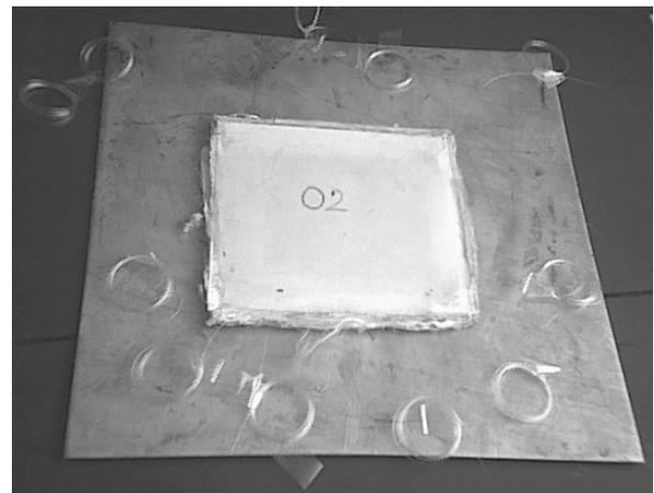
Figure 3. Photo of the composite material specimen with the embedded optical fibers
