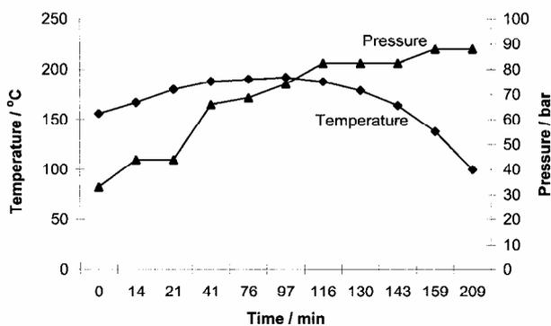
Figure 1. Optimal regime of laminated composite material hot-pressing
