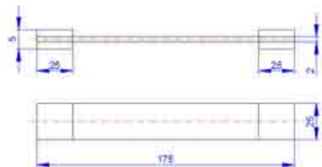
Figure 3. Specimen for the tensile investigation perpendicular to the direction of fibres ("transverse specimen")
