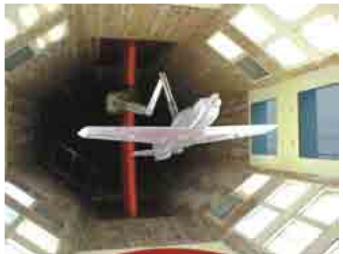
Figure 2. The LASTA-95 model on the model support system in the T-35 wind tunnel test section (front view)
