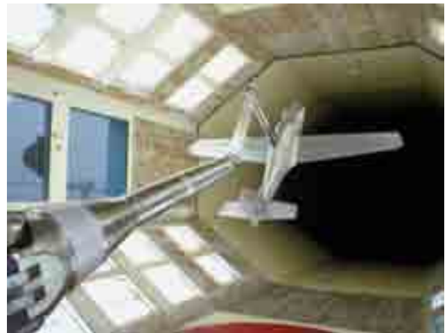
Figure 1. The LASTA-95 model on the model support system in the T-35 wind tunnel test section (rear view)
