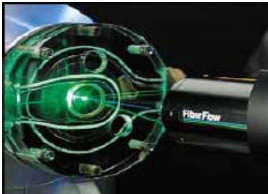
Figure 18. Investigation of the flow between the impeller blades of a pump (Grundfos A/S, Denmark) [6]
