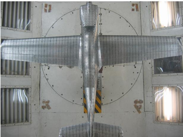
**Figure 14.** Flow visualization with cotton tufts in wind tunnel T-35 for flow with  $V = 100$  m/s [37]
