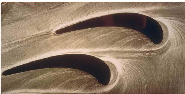
**Figure 17.** Oil flow visualization, airflow on the end wall of a turbine blade cascade. (Von Karman Institute) [15]
