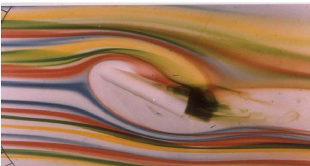
**Figure 6.** Water tunnel flow visualization by wall dye streaks. (Von Karman Institute [15])
