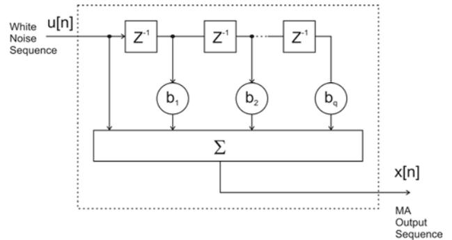
Figure 10. Model of the MA filter [7]
