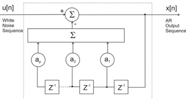
Figure 9. Model of the AR filter [7]
