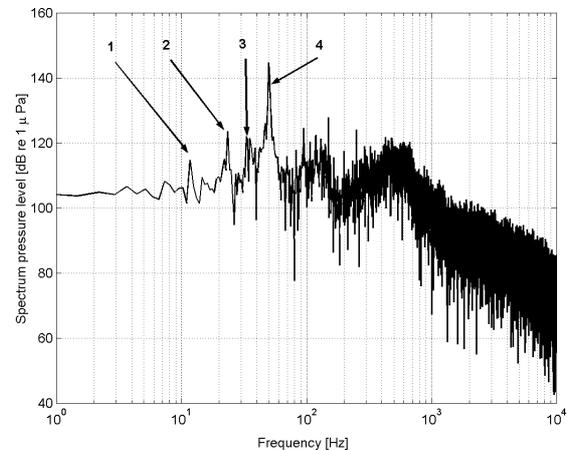
Figure 6. Spectrum of the hydroacoustic noise signal at CPA position
