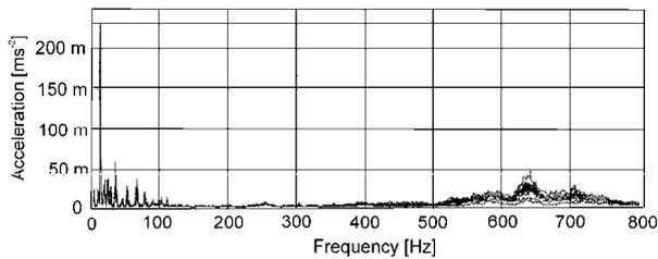
Figure 7. Vibration spectrum, vertical axis at ship's bow peak [6]
