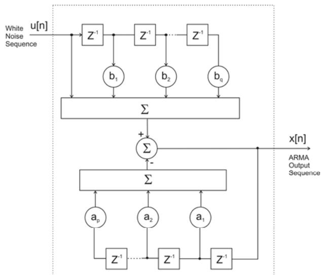
Figure 11. Model of the ARMA filter [7]
