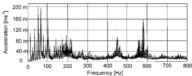
Figure 8. Vibration spectrum, vertical axis at home site of the main motor [6]
