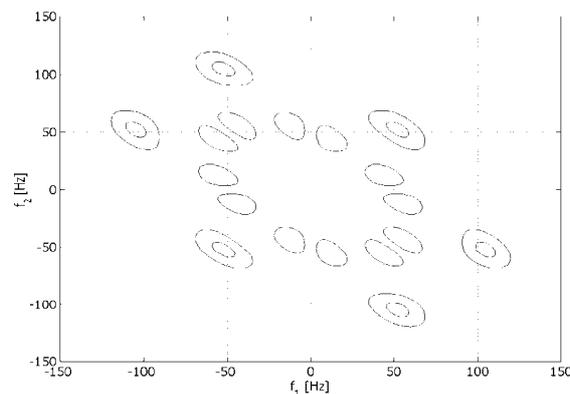
Figure 17. Bispectrum of the hydroacoustic noise signal when the CPA point is passed
