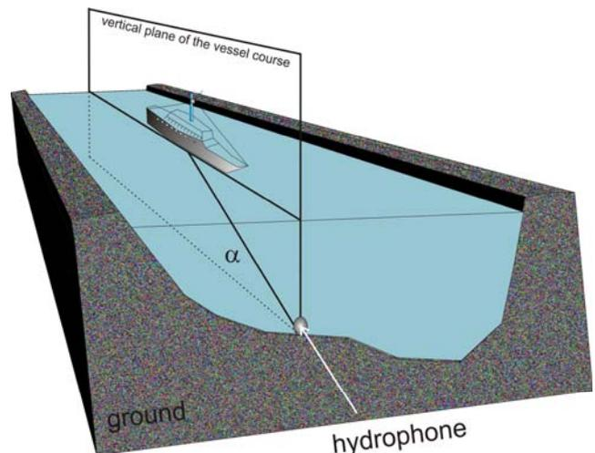
**Figure 3.** Hydroacoustic test range at the river
