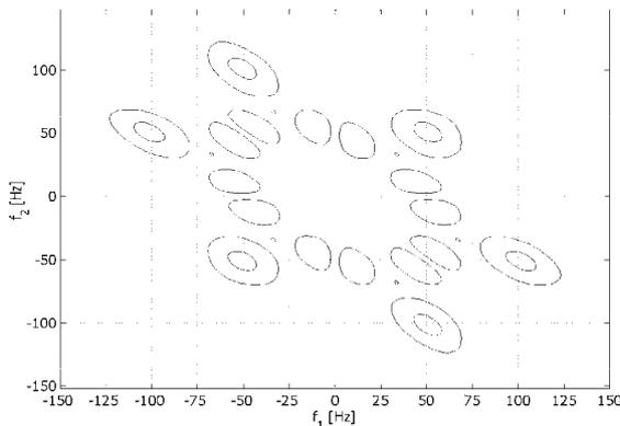
Figure 15. Bispectrum of the hydroacoustic noise before the CPA point is reached
