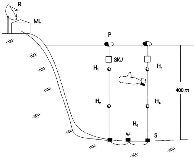
**Figure 1.** Scheme of the modern test range. ML – measuring laboratory, R – radar,  $H_1, \dots, H_5$  hydrophones, SKJ – communication unit, P – buoy [5].
