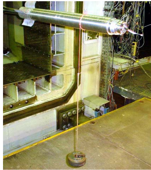
Figure 7. Calibration of one component transducer in the wind tunnel test section
