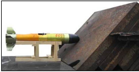
Figure 7. Detail of penetrability testing of shaped charge warhead in static conditions (BUMBLEBEE tandem warhead penetrability testing)
