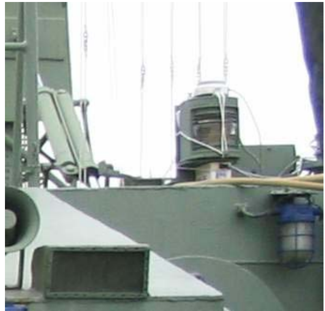
Figure 7. Location of the solarimeter for the solar radiation measurement and hygro-thermometer for exterior air humidity and temperature measurement
