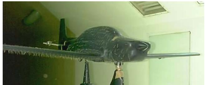
Figure 3. Flow visualization by tufts around the *LASTA-1* model [7]
