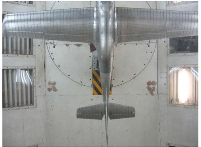
**Figure 10.** Flow visualization around the *LASTA-95* model at  $M = 0.3$ , angle of attack  $\alpha = 20^\circ$  and sideslip angle  $\beta = 0^\circ$  [4]
