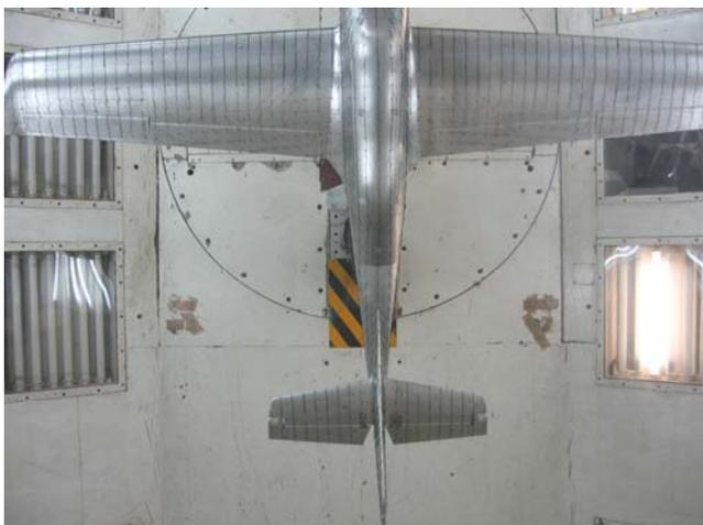
**Figure 9.** Flow visualization around the *LASTA-95* model at  $M = 0.3$ , angle of attack  $\alpha = 16^\circ$  and sideslip angle  $\beta = 0^\circ$  [4]
