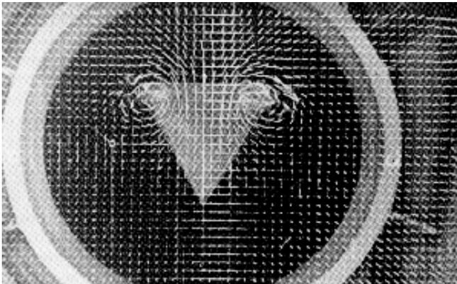
Figure 1. Flow visualization by tufts grid behind delta wing [1]
