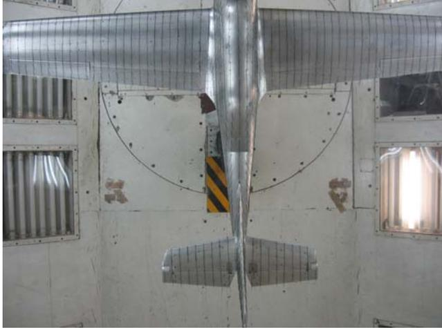
**Figure 7.** Flow visualization around the *LASTA-95* model at  $M = 0.3$ , angle of attack  $\alpha = 4^\circ$  and sideslip angle  $\beta = 0^\circ$  [4]
