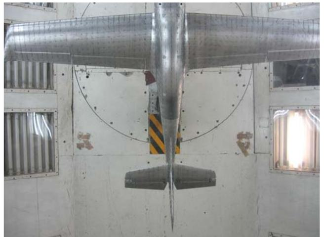
**Figure 11.** Flow visualization around the *LASTA-95* model at  $M = 0.3$ , angle of attack  $\alpha = 24^\circ$  and sideslip angle  $\beta = 0^\circ$  [4]
