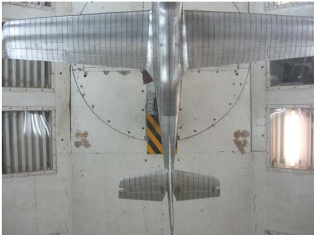
**Figure 8.** Flow visualization around the *LASTA-95* model at  $M = 0.3$ , angle of attack  $\alpha = 12^\circ$  and sideslip angle  $\beta = 0^\circ$  [4]
