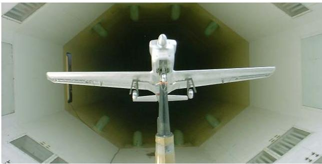
**Figure 4.** The *LASTA-95* model on the model support system in the wind tunnel *T-35* test section (front view)
