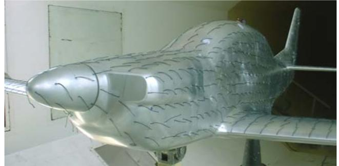
Figure 6. The model of *LASTA-95*, prepared for flow visualization [4]
