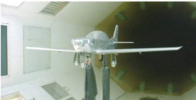
**Figure 5.** The *LASTA-95* model on the model support system in the wind tunnel *T-35* test section (side view)
