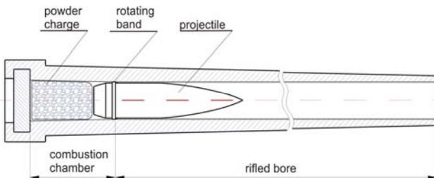
Figure 1. Illustration of a projectile in the weapon's barrel
