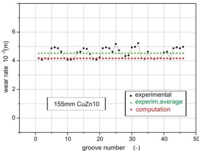
**Figure 6.** Illustration of rotating band cog wear for projectile 155 mm M107
