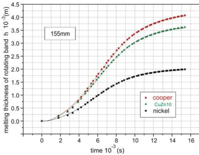
**Figure 4.** Diagram of changes of thickness  $h$  of the wear of layers for different materials in function of contact time duration
