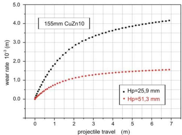
**Figure 7.** Diagram of rotating band cog wear with different rotating band widths for projectiles 155 mm M107 ( $H_p=25.9$ ) and M101 ( $H_p=51.3$  mm)
