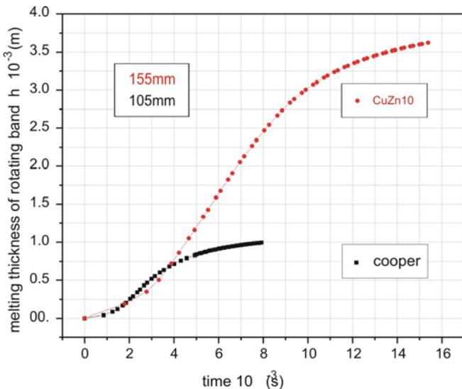
**Figure 5.** Comparative diagram of changes of the thickness  $h$  of the wear of layers in function of contact time duration for 105 mm and 155 mm systems
