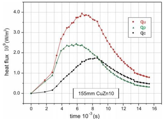
**Figure 3.** Diagram of the heating flux changes  $\dot{q}_u$ ,  $\dot{q}_c$ ,  $\dot{q}_p$  in function of contact time duration
