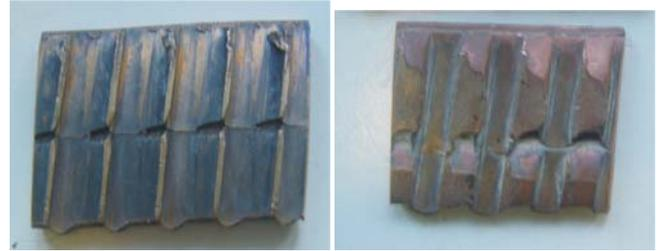
**Figure 2.** Illustration of the rotating band 155 mm (left) and 105 mm (right)
