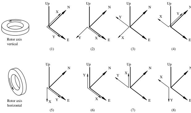
Figure 1. Eight position test sequence
