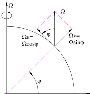
Figure 2. Earth rotation components
