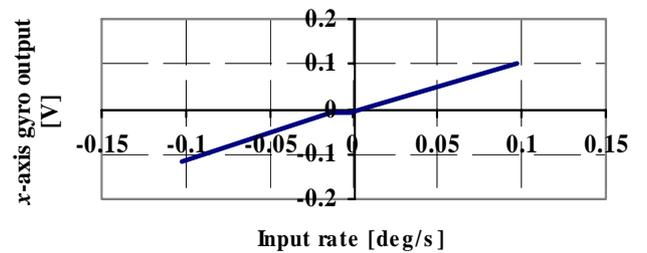
**Figure 3.** x-axis characteristic
