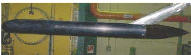
**Figure 1.** The axisymmetrical model in the test section of the T-38 wind tunnel
