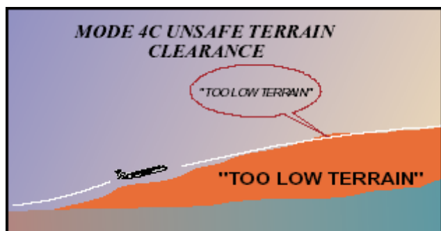
Figure 6. Unsafe terrain clearance, mode 4C
