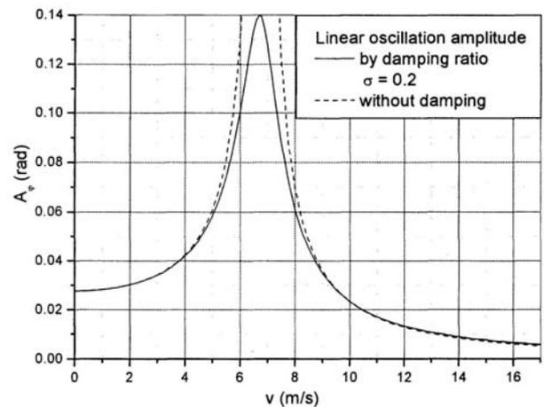
Figure 4. The relationship between the amplitude of the linear oscillations and the vehicle velocity, on wavy surface amplitude 0,05 m
