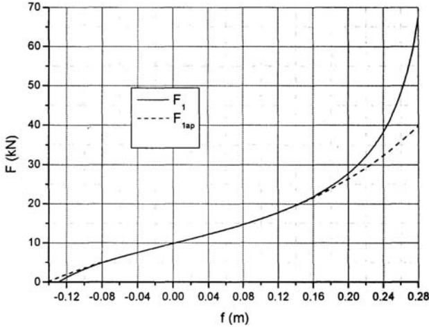
Figure 5. Suspension characteristics of the vehicle 1
