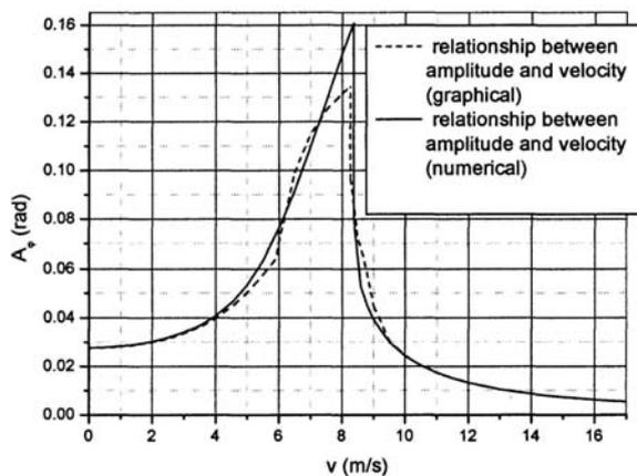
Figure 12. Numerical procedure of determination of the relationship between oscillation amplitude and vehicle velocity
