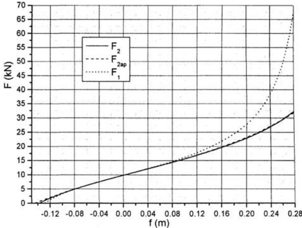
**Figure 9.** Suspension characteristics of the vehicle 2
