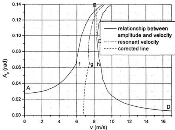
Figure 7. Relationship between the amplitude of the linear oscillations and the vehicle velocity on the wavy surface amplitude of 0.05 m
