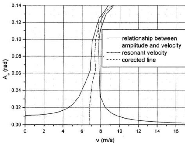
Figure 8. Relationship between the amplitude of the linear oscillations and the vehicle velocity on the wavy surface amplitude of 0.02 m
