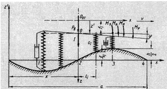
Figure 1. Tracked vehicle springs and dampers position on wavy surface
