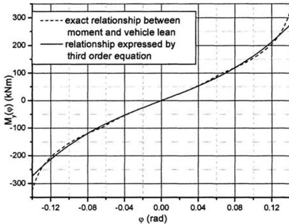
Figure 11. Approximation of the dependence of the torque on the vehicle 1 hull lean angle by third exponent equation
