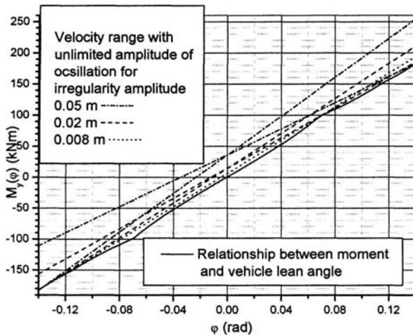
**Figure 10.** Dependence of the torque on the vehicle 2 hull lean angle
