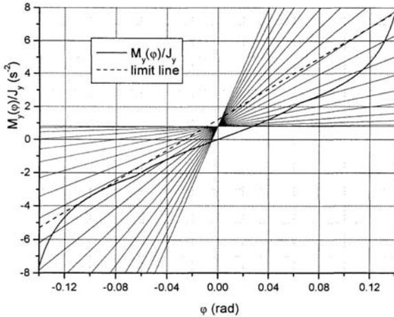
Figure 6. Graphical procedure determination of relationship between the amplitude of the linear oscillations and the vehicle velocity
