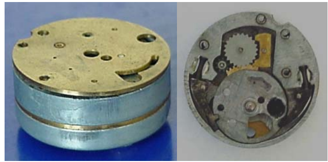
Figure 8. View of the realized design of safety arming device (left) and coupled gears train of the clock mechanism (right)
