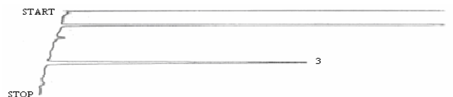
Figure 5. GC chromatogram of tri-EGDMA monomer standard solution Peaks (retention time, min): 1 = acetanilide (1.84 min), 3 = tri-EGDMA (6.66 min)
